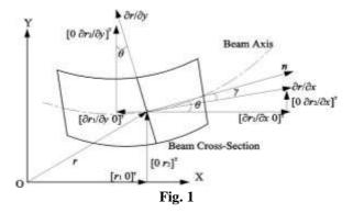
Research On Beam Deformation Based On Absolute Node Coordinate Method
